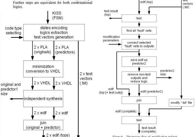
Figure 6. The process flow of modification and test
