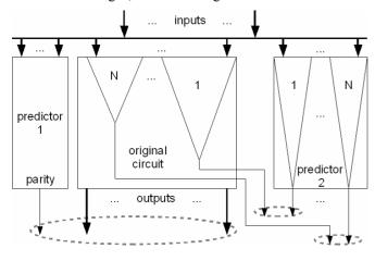
Figure 7. Block diagram of "Complete" design
