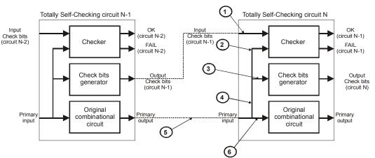
Figure 2. Proposed structure of TSC circuits implemented in FPGA
