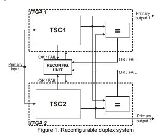
But this information is not sufficient to determine, which TSC circuit is wrong. Additional information to mark out the wrong circuit is generated by the original TSC circuit. The probability of the information correctness depends on the FS property and in many cases it is higher than 75%. In a case
