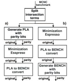
Fig. 7. Two different flows for creating a parity generator
