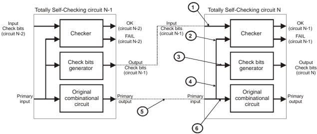
Fig. 8 Proposed structure of TSC circuits implemented in FPGA
