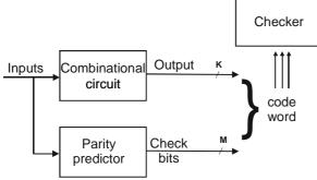
Fig. 1: Structure of a TSC circuit
