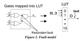
The original circuit has two inner nets. The original set of the test vectors covers all faults in these inner nets. These test vectors are redundant for an LUT. For circuits realized by LUTs a change (a defect) in the memory leads to a single event upset (SEU) at the primary output of the LUT. Therefore we can use the stuck-at fault model in our experiments to detect SEU – only some of the detected faults will be redundant.
