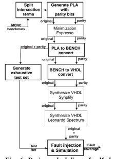
Fig. 6. Design scheduling of self-checking circuit
