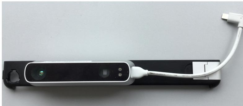
Figure 1.11: Structure Sensor with iPad frame and interface cable.
