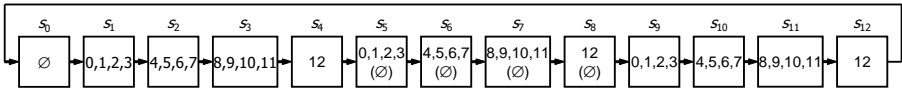
Figure 6.13: Evaluation of the terms in the stages of an optimized circular digit-serial multiplier with a distributed overlap (GCDO) for m = 13 and D = 3 . The values of the second indices j of the terms T_{i,j} are introduced. Multiplication logic is switched off in stages s_5 through s_8 in the first and last clock cycles (denoted by \emptyset ). Multiplication takes q = 5 clock cycles.
