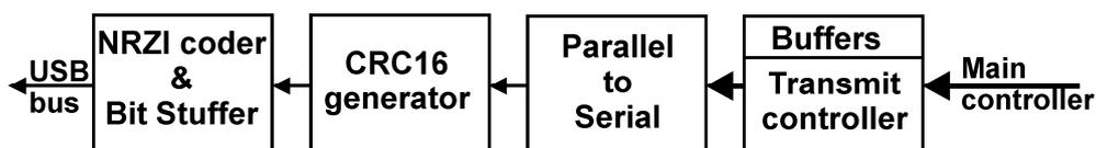
Figure 3: Transmitter block diagram
