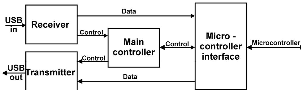
Figure 1: USB core block diagram
