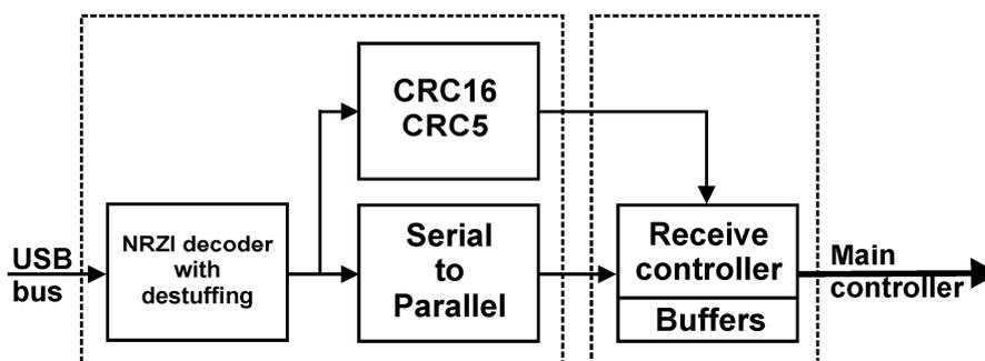
Figure 2: Transceiver block diagram
