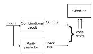
Figure 4: The on-line diagnostics design
