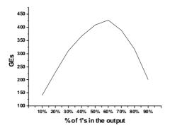
Figure 6. Dependency of the area overhead on the ratio of output '1's
