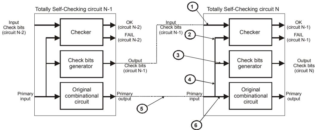
**Figure 3. Proposed structure of TSC circuits implemented in FPGA**
