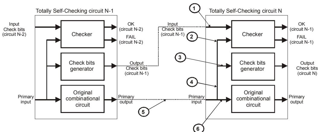
Figure 2. Proposed structure of TSC circuits implemented in FPGA
