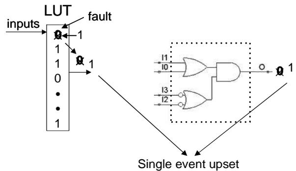
Figure 3. Fault Model – Example
