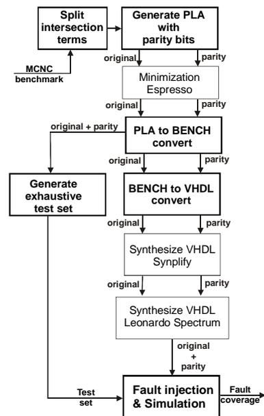
Fig. 6. Design scheduling of self-checking circuit
