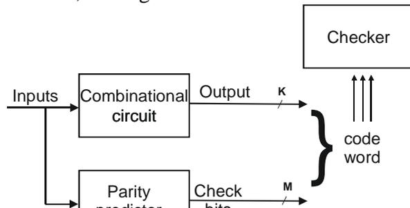
Fig. 1: Structure of a TSC circuit
