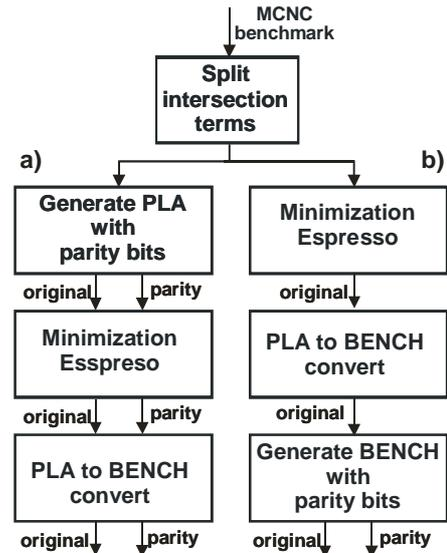
Fig. 7. Two different flows for creating a parity generator
