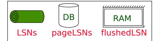
Each log record has a unique Log Sequence Number (LSN). Log records flushed to disk - LSNs always increasing. Each data page contains a pageLSN. - The LSN of the most recent log record for an update to that page. System keeps track of flushedLSN. pageLSN The max LSN flushed so far. Log tail" in RAM WAL: Before a page is written, - pageLSN  $\leq$  flushedLSN
