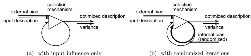
Figure 3: An iterative design tool sensitive to hidden details
