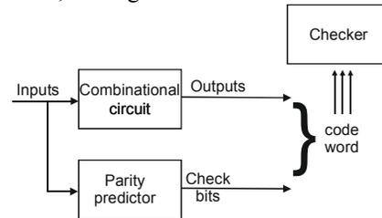
Figure 1: The self-checking circuit design
